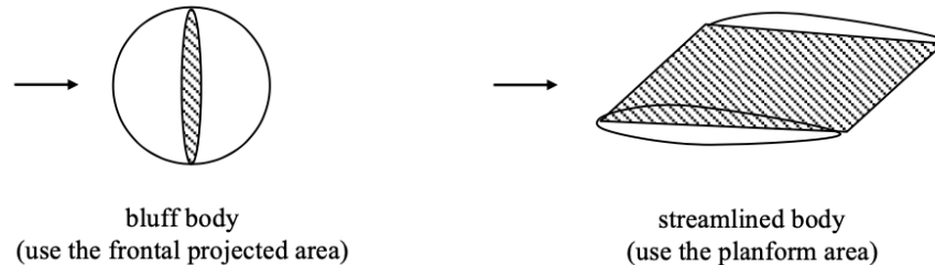
FIGURE 9.28. Illustrations of the frontal projected area (left) and the planform area (right).
