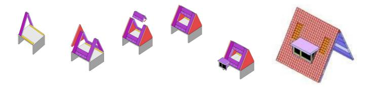
The benefit of this systemconstruction is that sizes are standardized (modular sizes a multiple of 150 mm) it provides flexibility during the building phase, consumer: "on second thought, we do want a dormer ..." and as an extra benefit the inhabitant can remove an element and order an element complete with sky light or a dormer without any need for sawing or cutting. Isn't it easy?
