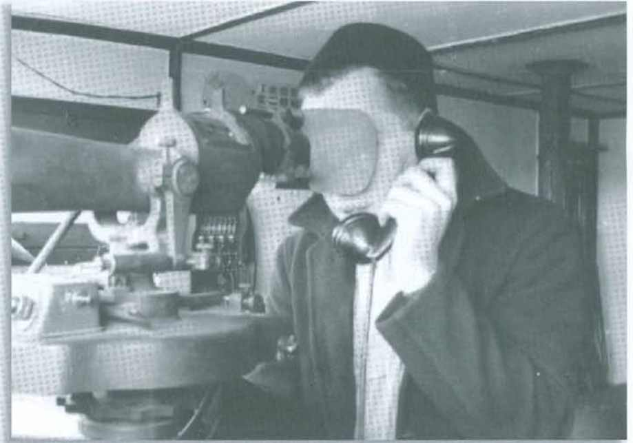
Azimuth instruments were used to measure target direction in a horizontal-based position finding system. (Alaska State Parks, Chuck Underwood Collection)
