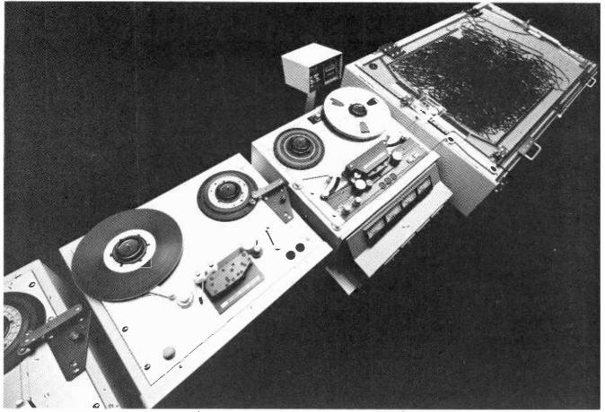
The 16:1 system is specially designed for medium-scale cassette duplicating. Up to 300 C-30s, for instance. Thanks to the latest full-modular concept, it meets your specific need exactly and economically.
