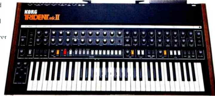
● DIMENSIONS: 1012(W) · 173(H) · 524(D)mm ● WEIGHT: 23.5kg ● ACCESSORIES: Connection Cord, Memory, Cassette, Dust Cover, Foot Switch, 6.1
