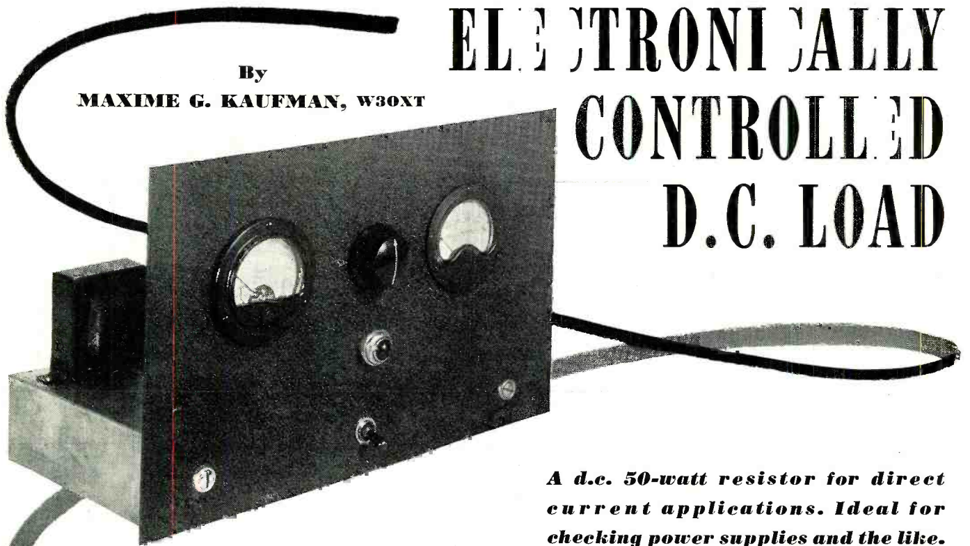
Panel view of home-built unit. Meters indicate both voltage across and the current through the load.
