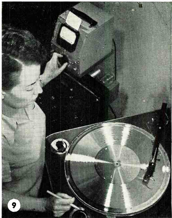
Technician making sound test of the metal "mother" recording.
