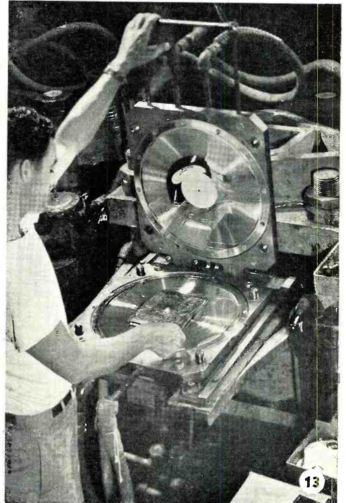
The surface of the "stamper" being hardened by chrome plating.
